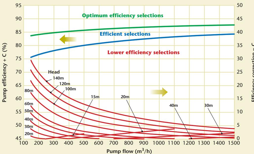
**Figure 8:** Efficiencies of double entry axially split casing pumps at 1450 rpm.
