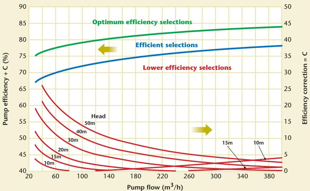
**Figure 4:** Efficiencies of end suction pumps with their own bearings at 1450 rpm.
