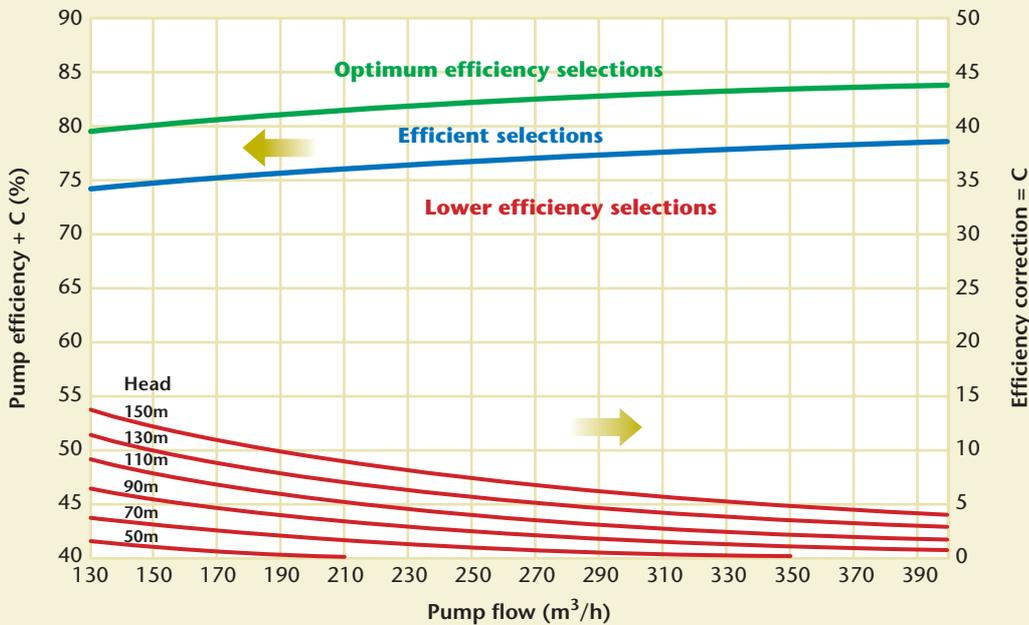
**Figure 7:** Efficiencies of double entry axially split casing pumps at 2900 rpm.
