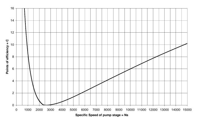
Fig 9. Plot to determine value of C
