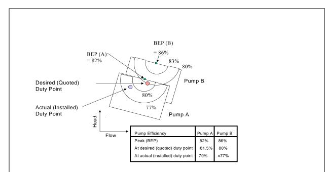
A user requests quotes for a pump at a particular desired duty. Manufacturers A and B offer the pumps shown, which are the best that they can offer from the ranges that they have. (These two pumps are excerpts from two manufacturers' ranges of the type shown in Fig 6).
