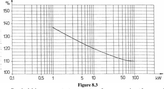
Required driver power output as percentage of pump power input for range of application from 1 to 100 kW
