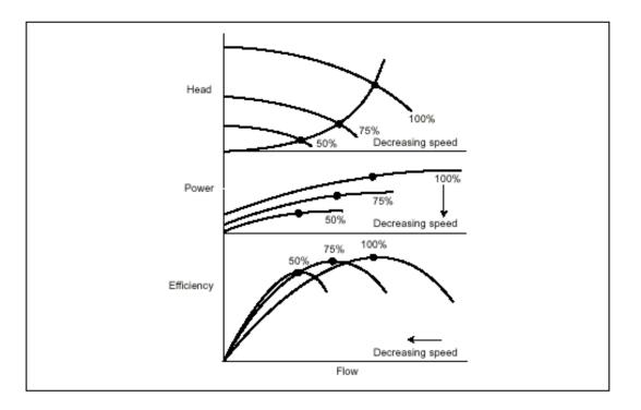
Fig 7. Effect of speed reduction on pump characteristics
