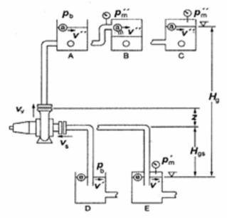
Figure 8.1 Pumping system with various arrangement in <u>negative NPSH</u> operation
