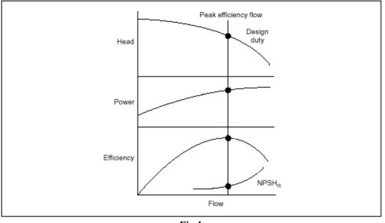
Fig 1. Pump characteristics
