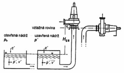
Figure 8.4 *NPSHA*\_examination in suction mode for horizontally and vertically installed pump
