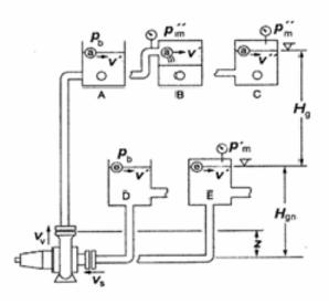
Figure 8.2 Pumping system with various arrangement in <u>positive NPSH</u> operation
