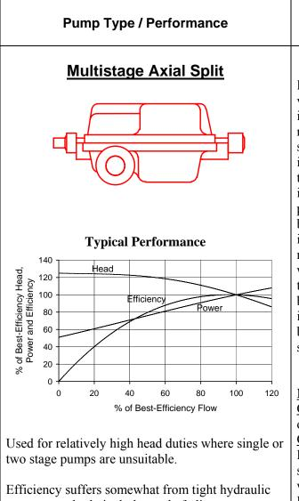
passages and relatively large shaft diameter at impellers. Also from larger wear ring clearances on hot pumps.
