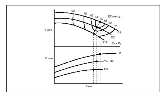
Fig 4. Pump characteristics showing various impeller diameters
