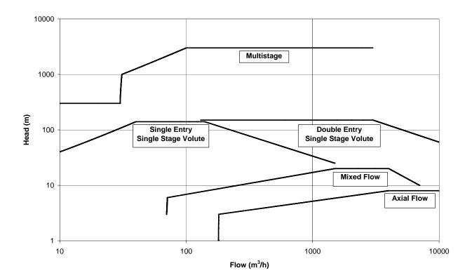
Fig 5. Indication of head and flow coverage of basic pump types
