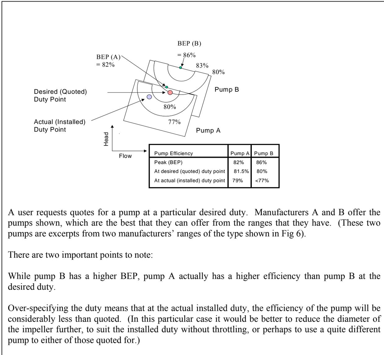
A user requests quotes for a pump at a particular desired duty. Manufacturers A and B offer the pumps shown, which are the best that they can offer from the ranges that they have. (These two pumps are excerpts from two manufacturers' ranges of the type shown in Fig 6).
